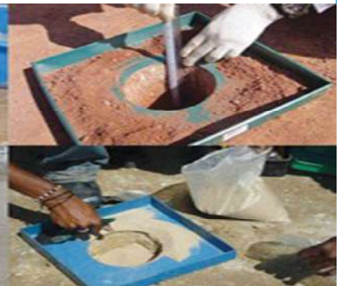
फोटो : Quality control of Compaction - sand replacement test
