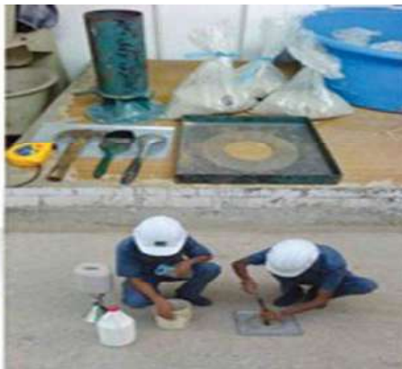
फोटो : Quality control of Compaction - sand replacement test
